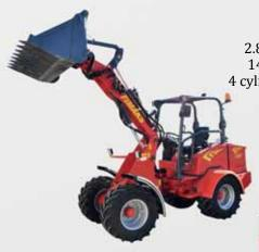
2.8 meters lifting height 1400 kg lifting capacity 4 cylinders Perkins engine 50 HP/37 kW power 0-20 km/hour speed
