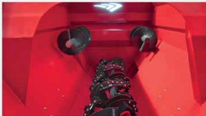
4 and 6 cubic meter horizontal mixer feeders internal mechanism look.
