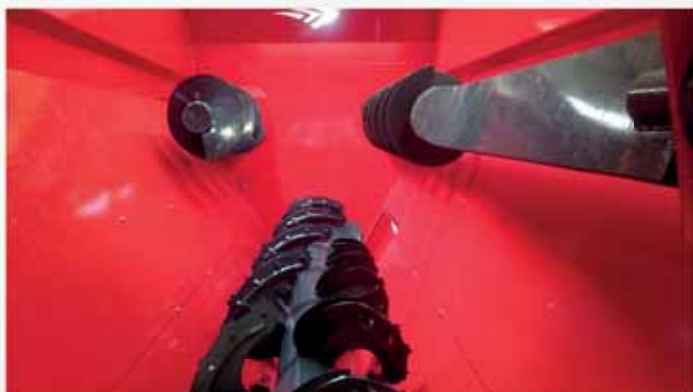
9 and 12 cubic meter horizontal mixer feeders internal mechanism look.
